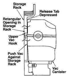
Lower the vac until the upper vac hook and lower hook are engaged and the bottom of the vac canister rests on the rack. The release tab will pop out over top of vac.
